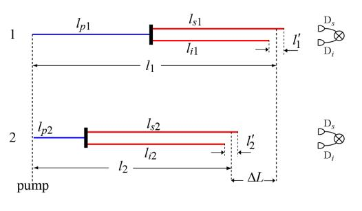
$$R_{si} = C[1 + \gamma' (\Delta L') \gamma (\Delta L) \cos(k_0 \Delta L)]$$
